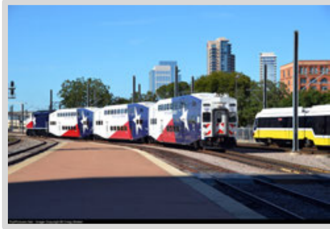
Image 4.7: The Trinity Railway Express in Downtown Dallas, an example of commuter passenger rail. The TRE service operates between Downtown Dallas and Downtown Fort Worth and makes 10 stops along its 30 mile route. The advertised one-way travel time is 1 hour for an average speed of 30mph. In a more suburban or rural setting, commuter rail would make fewer stops and be able to travel up to 79 mph. Commuter rail is one possible service option that could be recommended by the Texas Oklahoma Passenger Rail Study.
