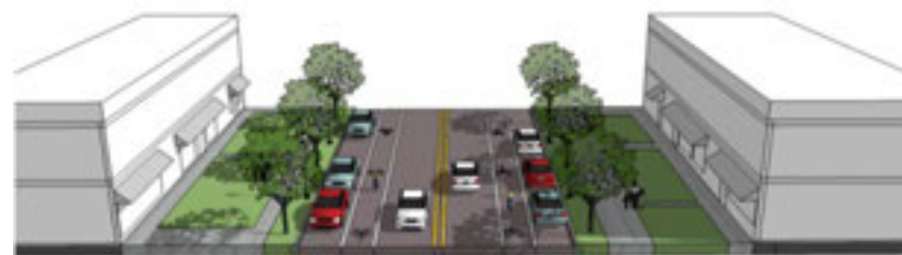
Image 4.2: Two-Lane Urban Collector. Urban Collectors typically include one lane for through motor vehicle traffic in each direction with parallel or angled parking. Turn lanes and bicycle lanes are optional based on the existing right-of-way constraints and the context of the street. The sidewalk corridor nearly always includes a paved furniture zone where trees in tree grates, light poles, and other street furniture are placed. The sidewalk corridor is often wider than other thoroughfare types, taking up more of the available right-of-way.
