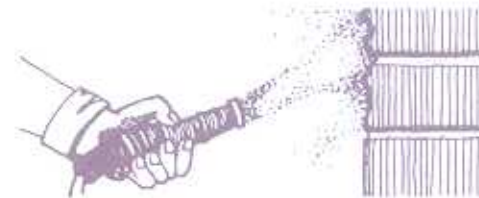
Sandblasting is never recommended because it can damage or corrode the building surface.
