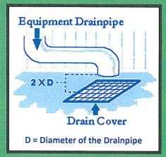
Notice that the very bottom of the equipment drainpipe is above the top of the sewer/drain/septic line. This ensures that any back flow will not enter into the equipment through the drainpipe. The vertical distance between the drainpipe and the flood level rim should be two times the diameter (2 X D) of the drainpipe, but never less than one inch. Here are some examples of incorrect air gaps:
