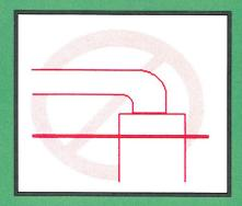
Note that having an 'exit valve' (see middle illustration above) installed in a drainpipe does not count as an air gap. This 'valve' may easily become clogged enough to allow sewage to continue traveling up the drainpipe.
